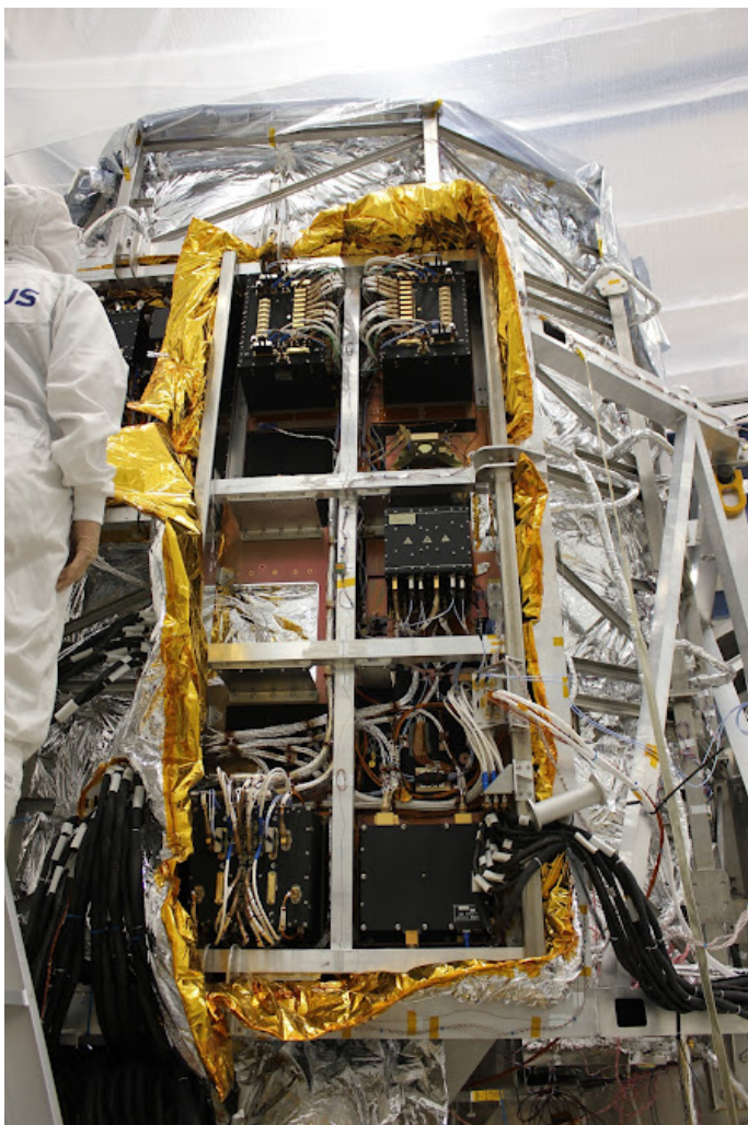
Fig. 14. NISP Warm Electronics: the identical DPUs can be seen on the top of the picture, while the ICU is located at the centre (right) of the so-called Spacecraft Y panel. Image courtesy Airbus Defence and Space
