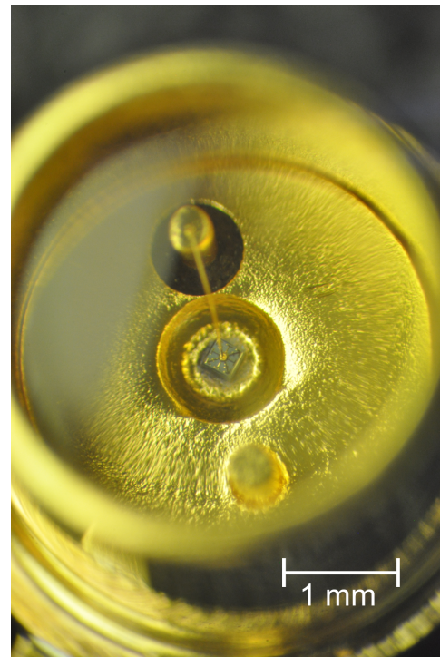
Fig. 2. Closeup of finished LED: wire-bonded semiconductor die (centre), inside gold-coated housing, behind hermetically sealed glass (image courtesy of von Hoerner & Sulger ).
