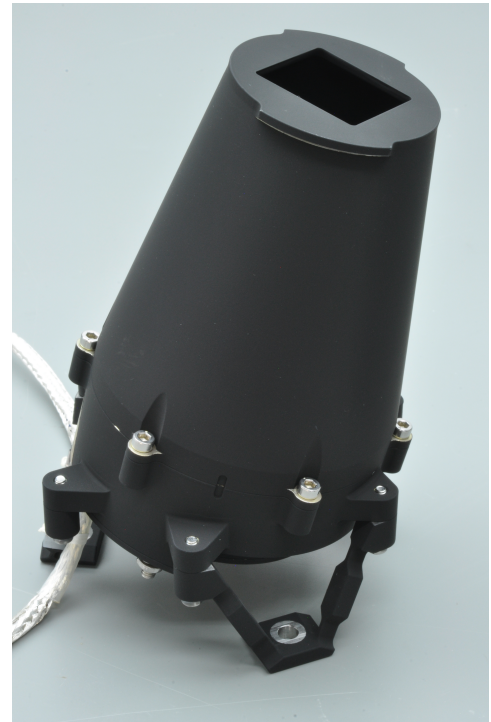
Fig. 8. NI-CU flight model before integration into NISP. The beginning of the ~680 mm nominal and redundant harnesses are visible at the bottom left, connecting to a long harness to the warm electronics at a connector bracket on the NISP structure. Despite being located far outside NISP's optical beam, it is fully coated with black PNC. Only screws and harness remain uncoated.
